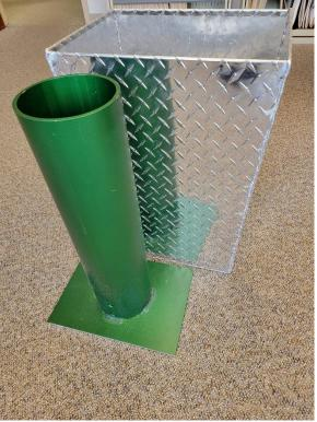
Flotec's Oxygen Cylinder Fill Pot provides for a vertically directed release of high-pressure gas in the event of cylinder rupture during cascade transfilling. Manufactured from the highest quality materials, our fill pots employ a solid water jacket barrier between the inner cylinder shell and outer casing.
